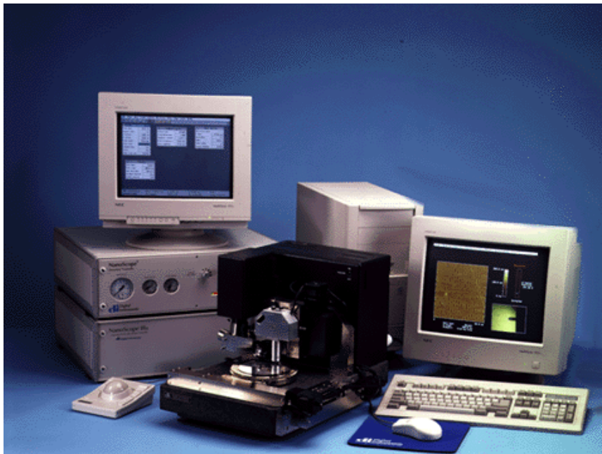
Figure 2. The Dimension 3000 AFM is capable of accommodating large samples and a fluid cell.
