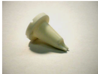
Figure 14. Alumina Kinematic Head
