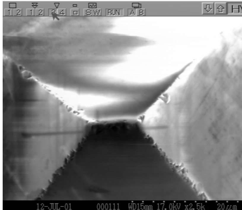
Figure 5 SEM micrograph of the probe tip used on Polaris . The view is essentially from the vantage point of a part being probed. The 10\ \mu\text{m} long cylindrical contact is oriented vertically in the machine.
