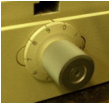
Figure 24: An adjustable slide base was used to determine the peak locations on either end of the liner.
