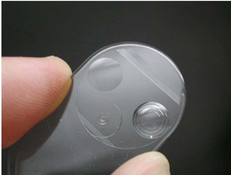
Figure 1. Example of Lens Fabricated from Injection Molding
