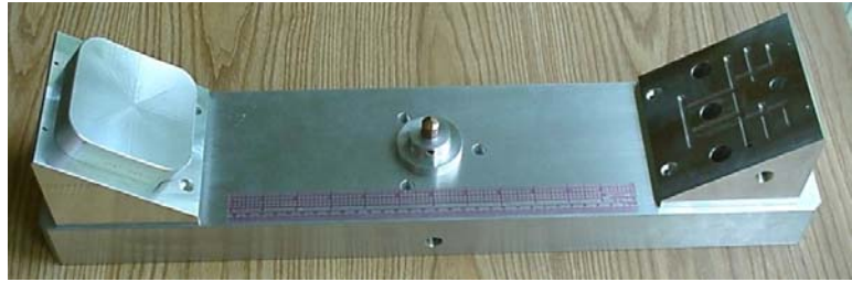
Figure 4. Alignment Fixture Showing Center Plug and two vacuum pedestals, with mirror blank mounted on left
