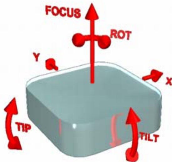
Figure 2. The four degrees of freedom in positioning an optical part
