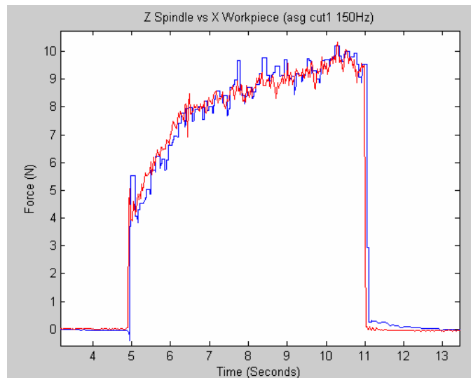
Figure 14 Comparison of the cutting forces measured on the work piece and spindle
