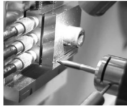
Figure 2: Workpiece mounted on three-axis piezoelectric load cell
