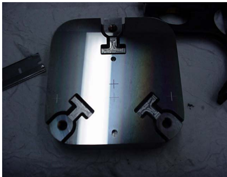
Figure 3. Diamond flycut back surface of M4 showing the four alignment crosshairs and three part mounts
