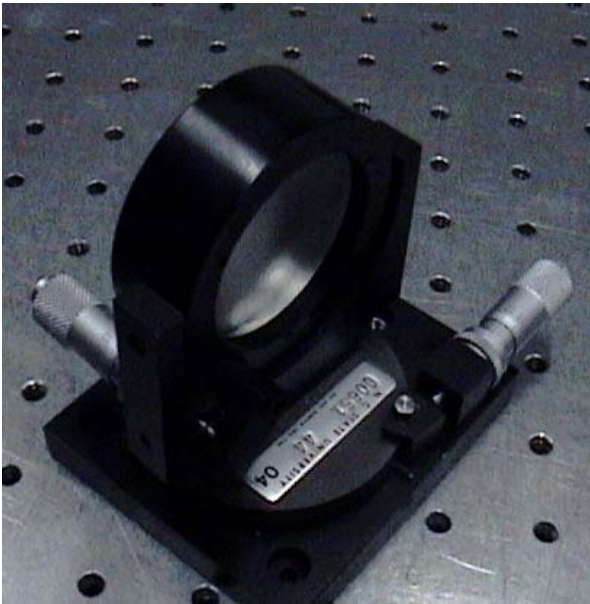
Figure 1. Optical alignment fixtures are not suitable for fixturing parts for fabrication.
