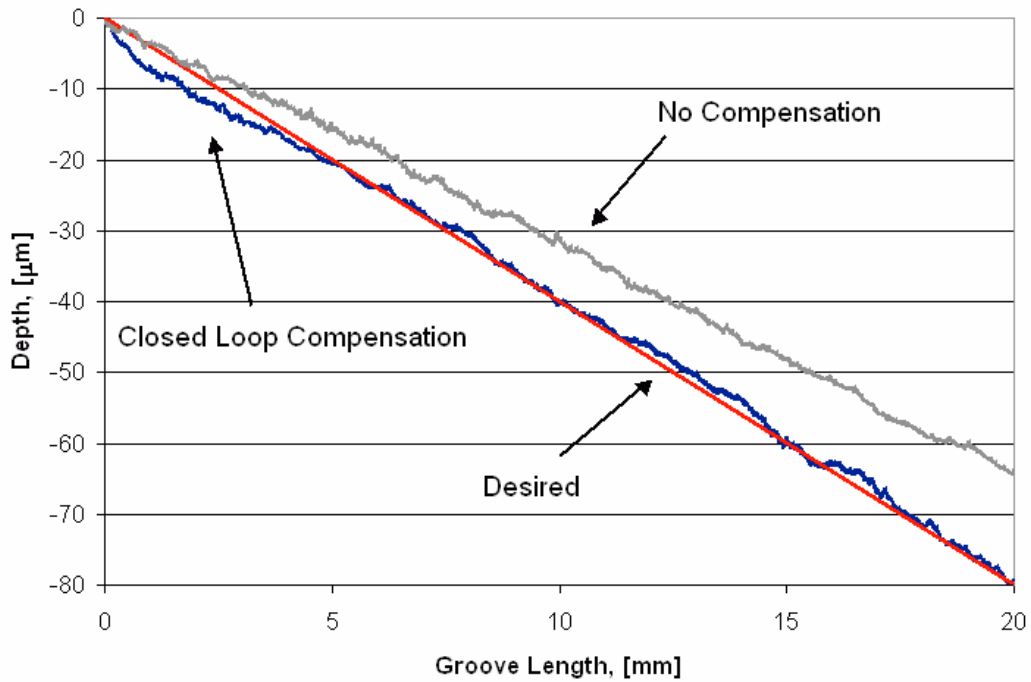
Figure 9. Desired, Spindle Feedback and No Compensation Profiles, Tilt = 30°, Depth = 0-80 mm, Upfeed = 10 mm/rev, Spindle Speed = 10,000 rpm, 4 mm long tool shank
