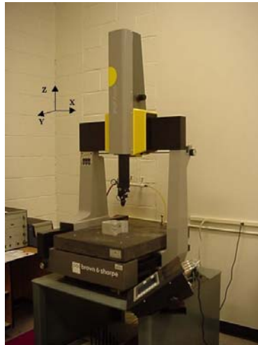
Figure 1. Moving bridge CMM at NCSU.
