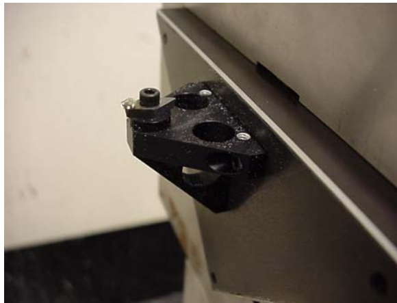
Figure 7. Tool holder and diamond tool mounted on the front of the triangular piston
