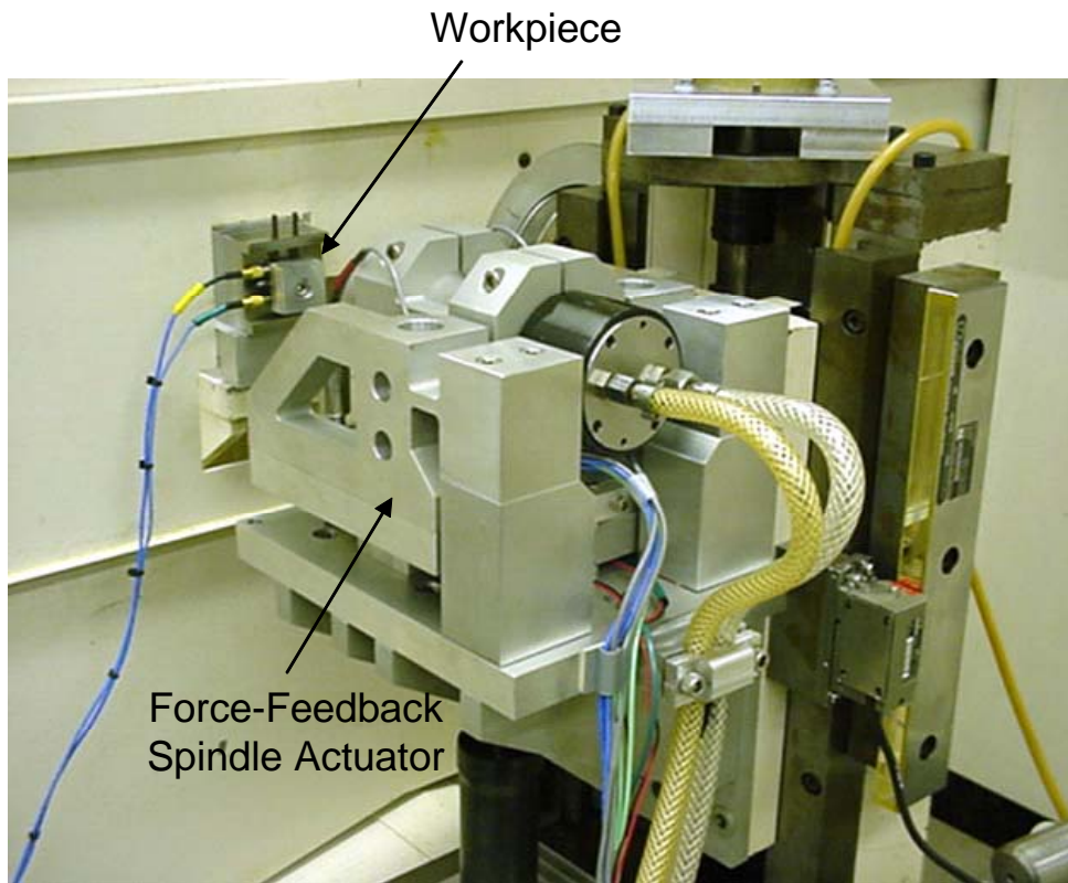
Figure 12. Force-Feedback Spindle Actuator mounted on Diamond Turning Machine
