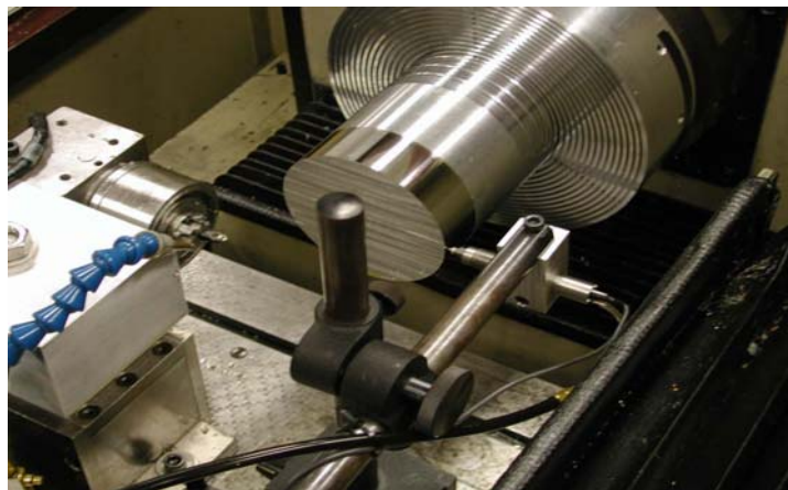
Figure 8. Experimental setup to machine swept sine wave on OD of cylinder and the air-bearing LVDT used to measure the final shape.
