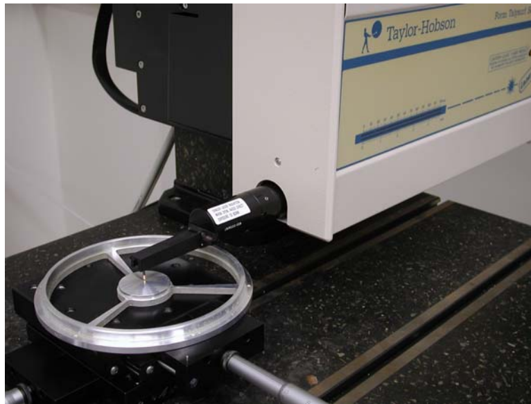
Figure 1. Taylor-Hobson Talysurf Profilometer with secondary mirror
