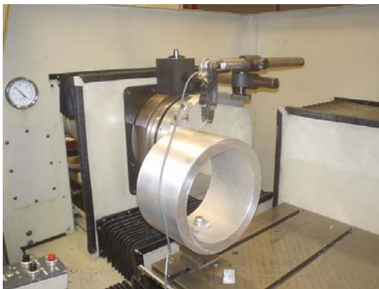
Figure 9. Tube mounted on a v-block is squared to the axes using an electronic indicator. The flycutter can be seen on the part spindle behind the tube.
