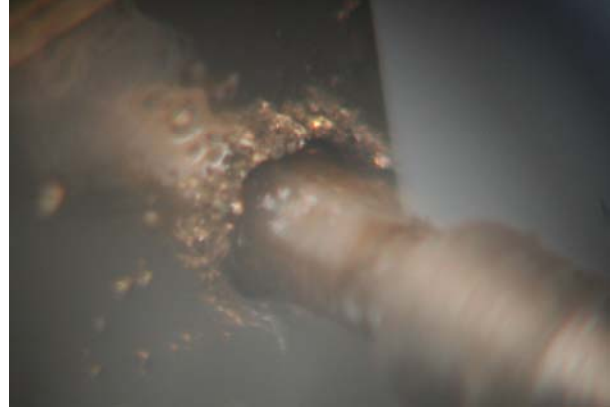
Figure 15. Closeup of pin hole being bored. View is through the on-machine microscope.
