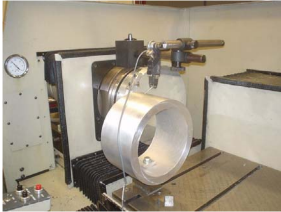
Figure 9. Tube mounted on a v-block is squared to the axes using an electronic indicator. The flycutter can be seen on the part spindle behind the tube.
