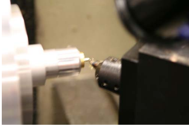
Figure 13. One of the brass pins being turned and the length measured.
