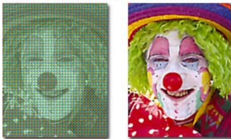
Figure 5. Raw Bayer pattern image (left) and interpolated image (right) of the same scene.
