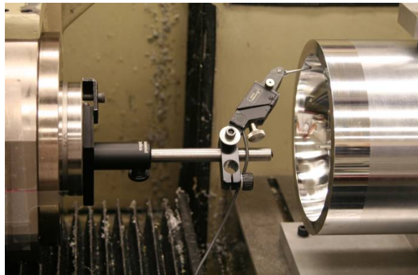
Figure 8: Radial Alignment of ID Chuck and Spindle
