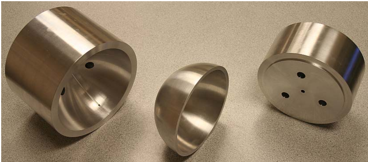
Figure 4. IC (left) and OC (right) vacuum chucks and unfinished hemishell (center).
