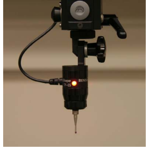
Figure 2. Renishaw TP6 CMM Probe.
