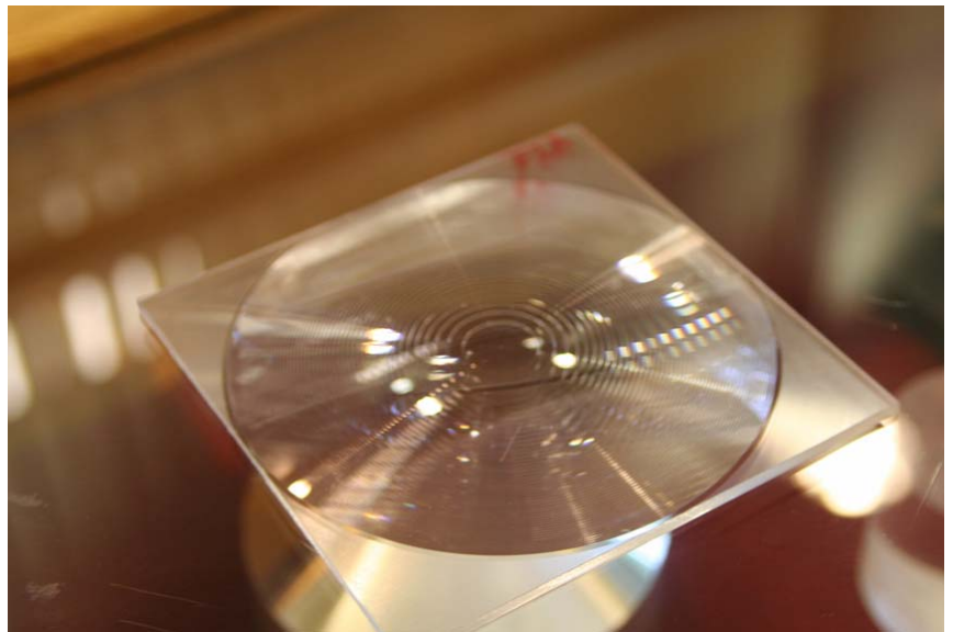
Figure 1. Finished aspheric groove PMMA Fresnel lens.
