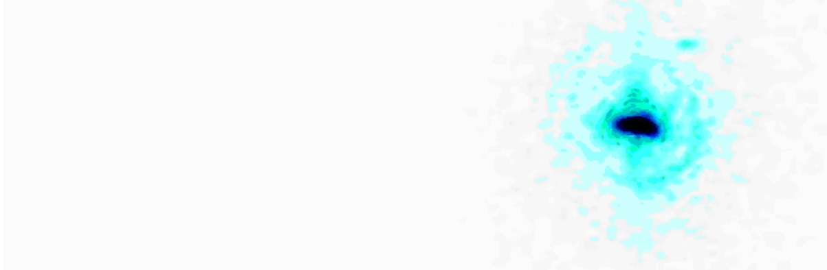
Figure 8. Spot formed by the center of the lens when illuminated with the large aperture beam shown in Figure 7. Images are shown as negatives for clarity.
