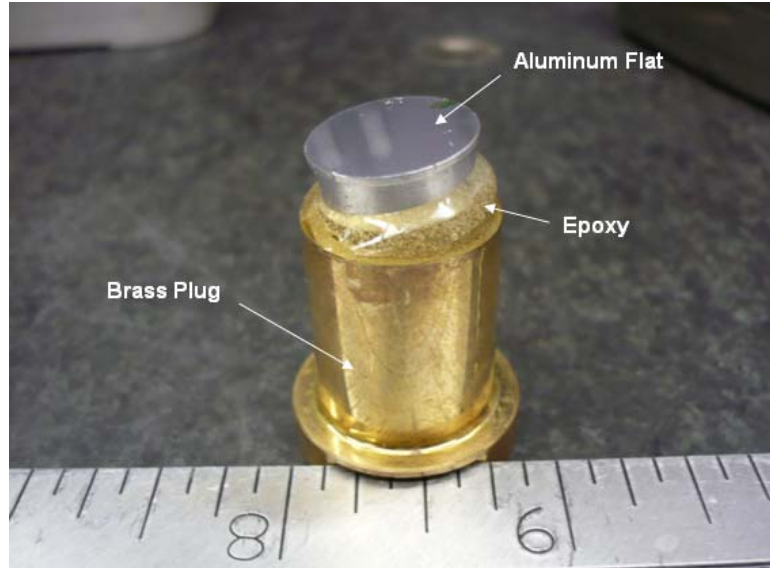
Figure 23. Tilted flat used for measuring \phi -axis to probe vertical alignment error
