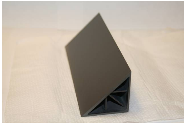
Figure 18. Actual FLORA II piston constructed by Coors Tek.
