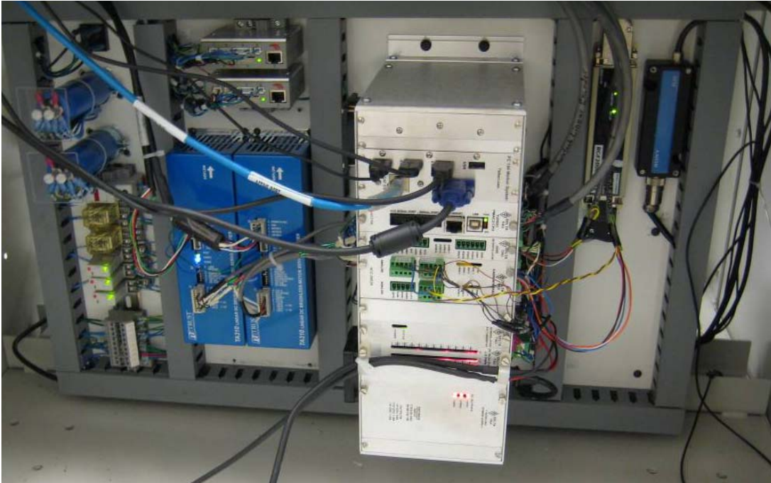
Figure 3. UMAC controller and Polaris 3D electronics.
