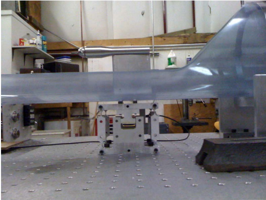
Figure 21. Thrust dynamometer with pulse jet engine mounted on airfoil shaped sting in the wind tunnel with the top of the wind tunnel removed for access to the engine.
