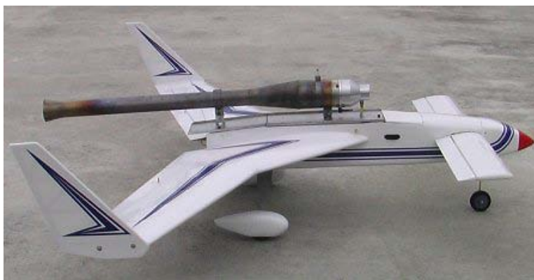
Figure 1. Hobby-scale, valved pulse jet mounted on a model airplane. Size is about 500 mm long and about 50 mm in diameter at the inlet section on the right. Thrust is about 20 N.
