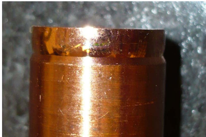
Figure 5. Copper test part of 12.7 mm nominal diameter. The toroidal region is approximately 2 mm wide at the top of the part.
