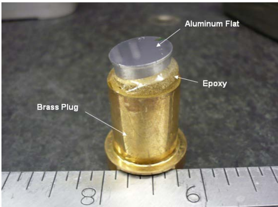
Figure 8. Tilted flat used for measuring y- alignment of probe to \phi -axis origin
