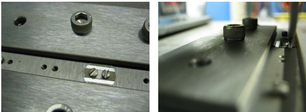
Figure 14. Photographs of the grinding process to create flexures on Inconel valves
