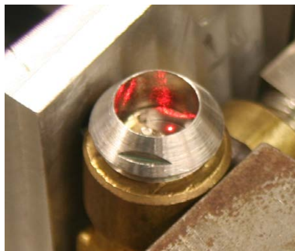
Figure 16. Closeup of the valve head showing the location of the laser spot on the valve.
