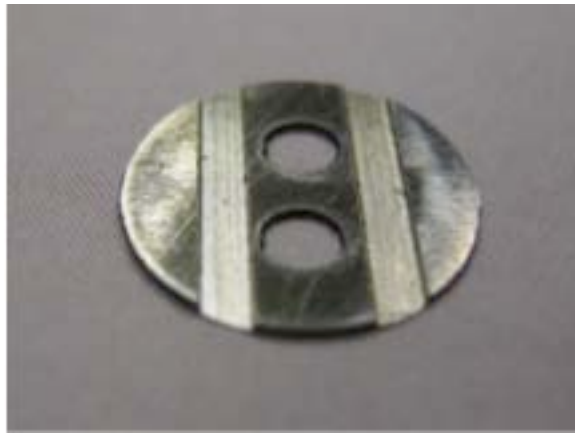
Figure 8. Photographs of the flapper valve designed for the small pulse jet engine. The material is heat treated Inconel with a pair of flexures ground to a thickness of 25 \mu\text{m} .
