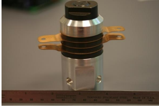
Figure 20. Image of BLT. Two aluminum masses bolted together with PZT material between.
