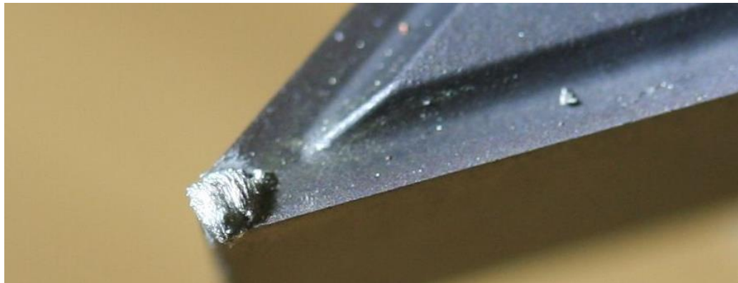
Figure 26. Photograph of Tool 2 after Turning an Overlapping Cut on 1199 Aluminum, Using a Feedrate of 22 mm/min Turned at 550 rpm at a Depth of Cut of 80 \mu\text{m}
