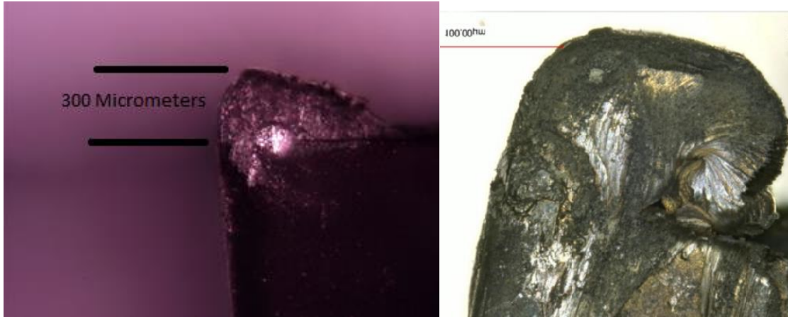
Figure 39. Side by Side Comparison of Built Up Edge Formed by Aluminum 1199 (L) and Plutonium Metal (R)
