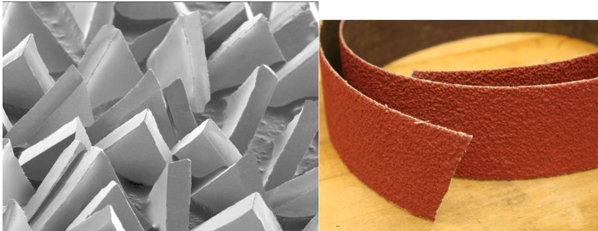
Figure 2. Alumina grits on coated abrasive. SEM image (left) [22], abrasive belt (right).
