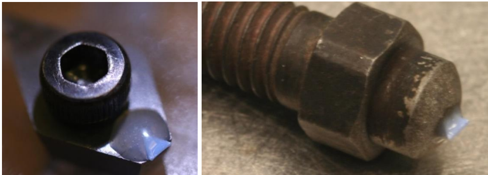
Figure 9. Epoxy mounting on a flat surface (left) and in a notched hole (right).
