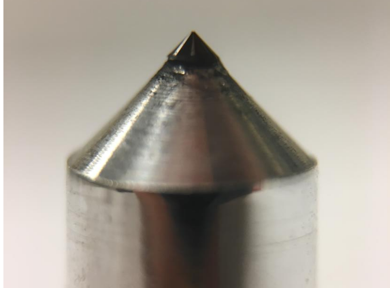
Figure 43. Diamond turned glassy carbon blank potted in an aluminum holder
