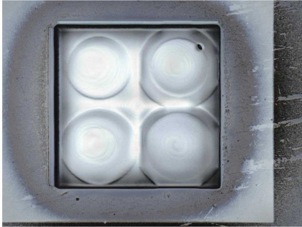
Figure 26. Features FIB milled with a 200 nm overlap
