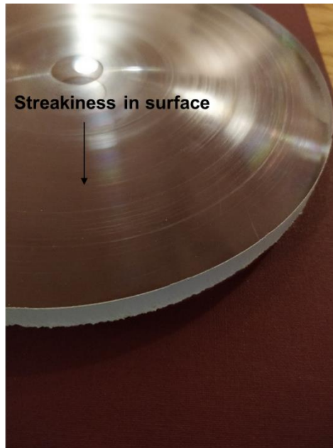
Figure 27. Polycarbonate after dry facing operation
