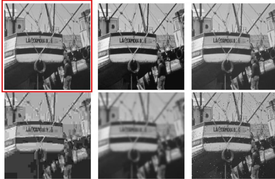
Figure 1. Deficiency of mean squared error for image comparison. The image in the red box (upper left) is the reference. The other images are clearly distorted but have identical MSE values.
