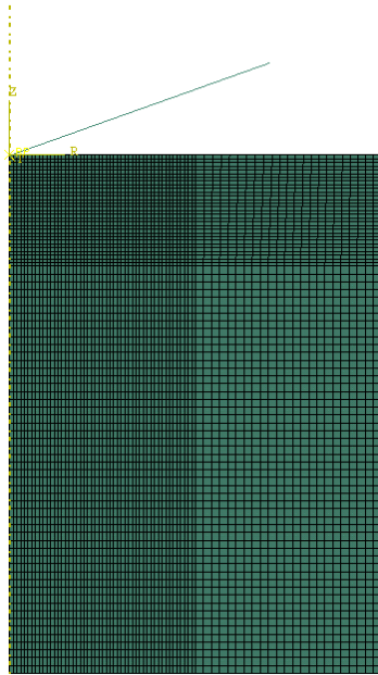
Figure 31. Mesh pattern used for the finite element model of the rigid spherical indenter and mold specimen
