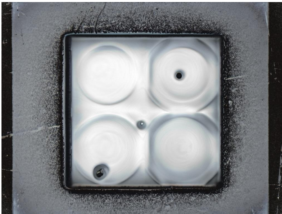
Figure 25. Feature FIB milled with a 100 nm overlap
