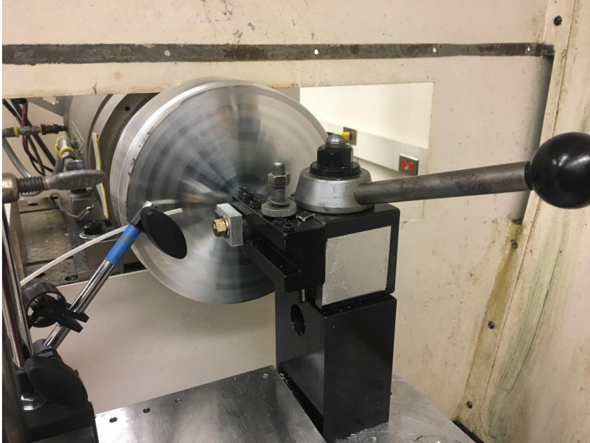
Figure 4-7: Diamond Turning Setup. Note the tube on the left side of the tool post.
