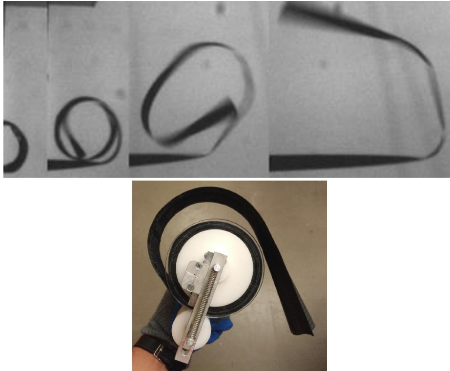
Figure 9-8 NCSU replicated the chaotic nature of a freely deploying boom in a one-G lab environment by suspending a boom vertically (top). Bottom image is a boom that is permanently deformed after long term storage due to creep and relaxation.
