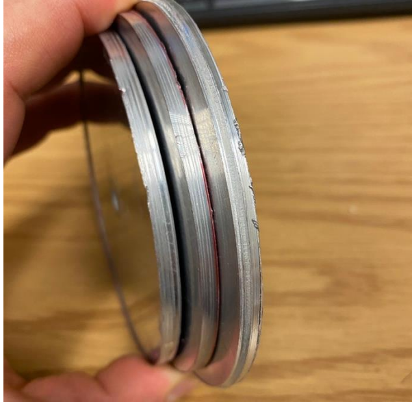
Figure 6-8: Cut edge of the aluminum alloy 1100 showing rough surface and built up material at the edge of the disc.
