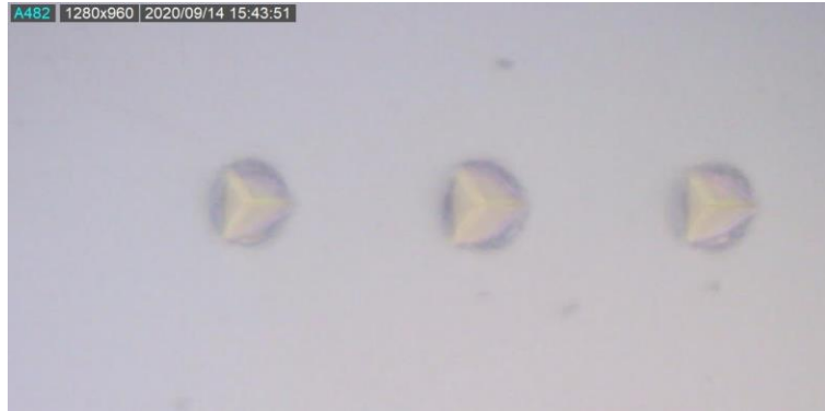
Figure 5.8. Three in-house Berkovich indents as viewed through a digital microscope.
