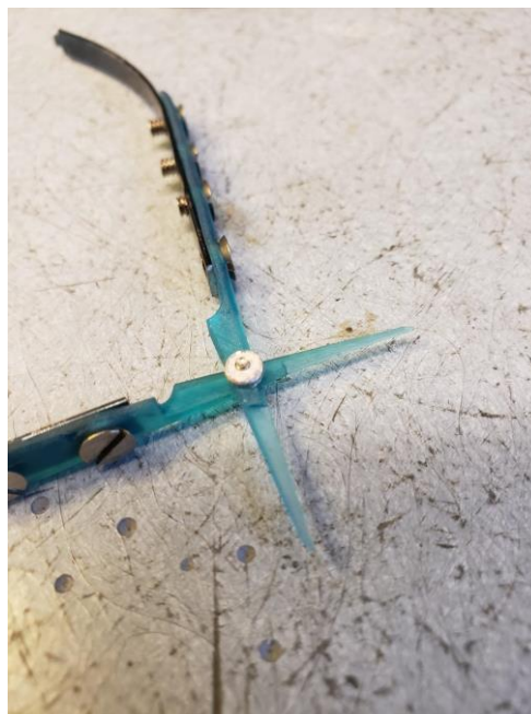
Figure 8-3. Blades of the 3D printed body for the device.
